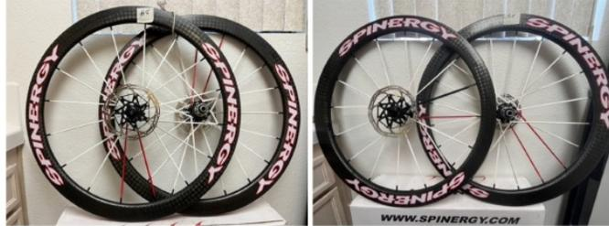
47 mm, carbon, Disc, thru-axle, 12x100, 6 bolts
